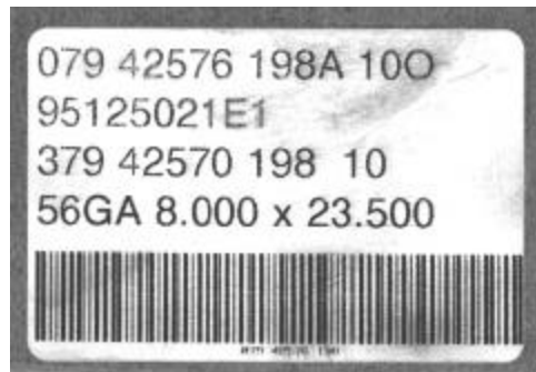
Figure 2 - Part label including part, assembly, and order number as well as dimensional information
