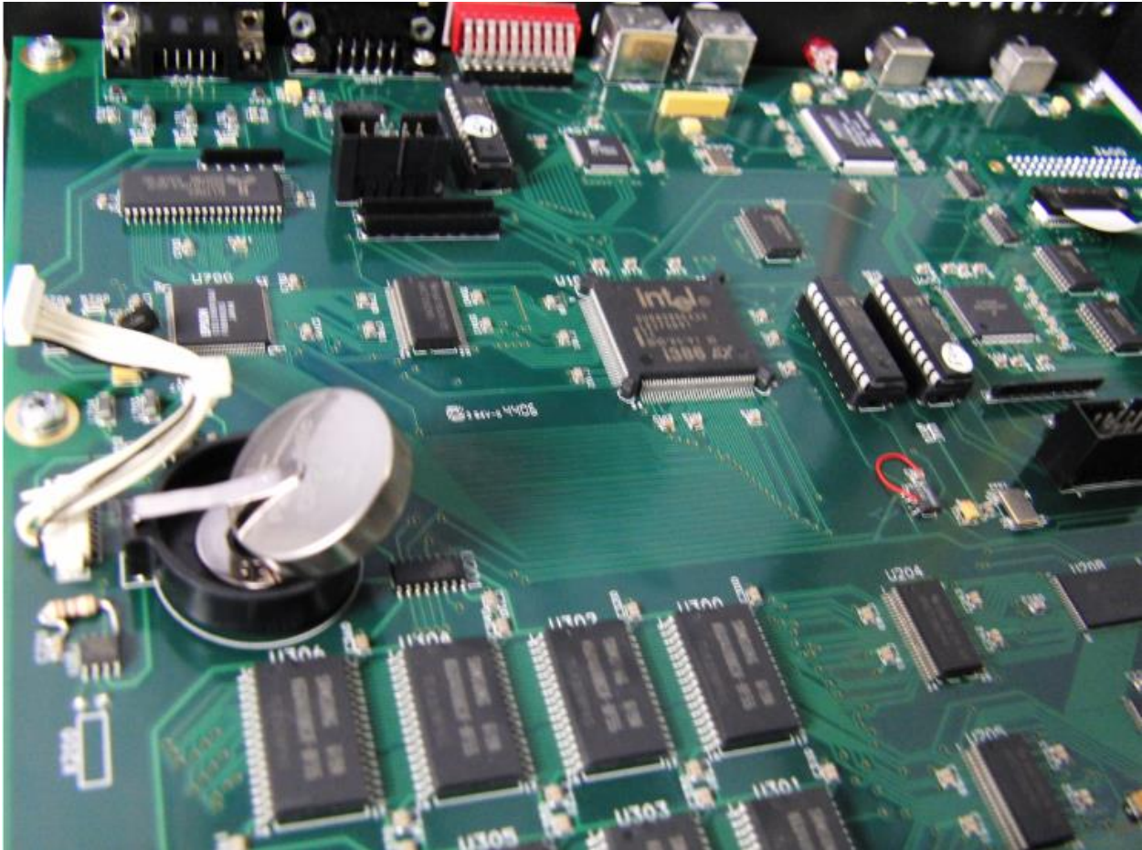
Figure 11 - Battery partially removed
