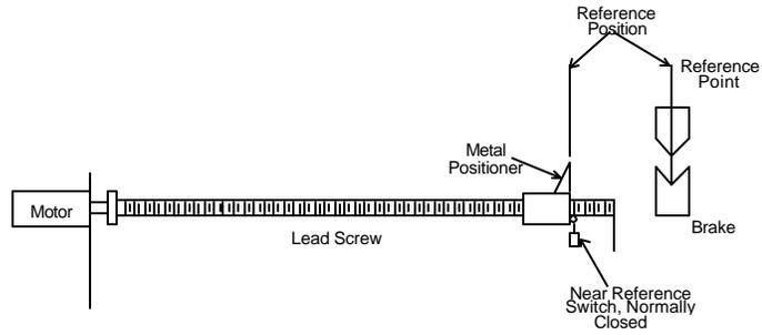
The switch for a NEAR REFERENCE MODE must be normally closed and remain open as long as the backgauge is on the switch or closer to the reference point than the switch. The switch for a FAR REFERENCE MODE must be normally open and remain closed as long as the backgauge is on the switch or farther away from the reference point than the switch.
