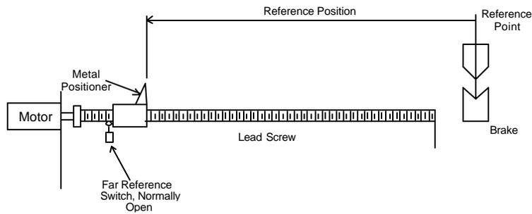
The controller will automatically reference itself when it is placed in the RUN mode. The reference is always achieved when the controller is moving in the forward direction. If a physical stop with a NEAR REFERENCE is used, the controller will reference itself when the gauge hits the stop going forward. If a physical stop with a FAR REFERENCE is used, the gauge will hit the stop in the reverse direction and then reference when the first forward encoder count is seen.
