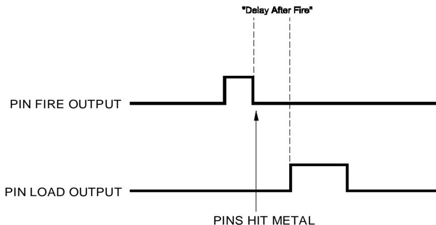
Figure 4-2 “Pin Fire” and “Pin Load” Timing
