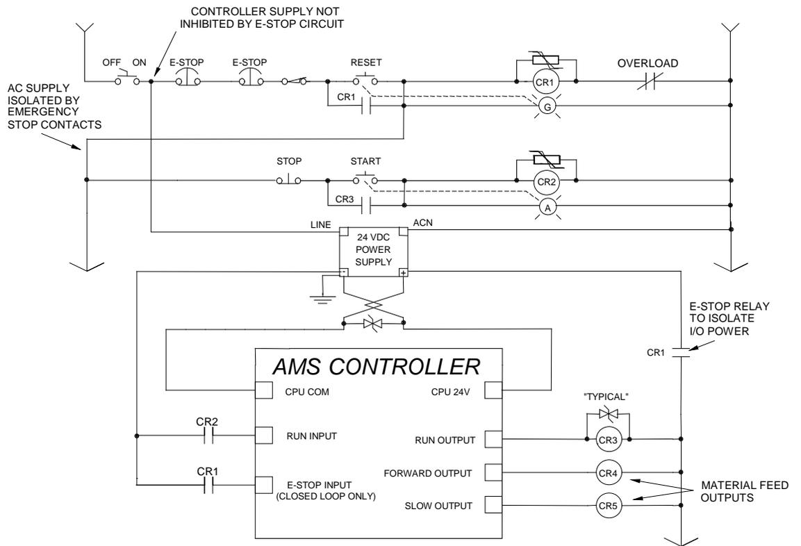
Figure 4-1 Circuit Example for Run and Estop
