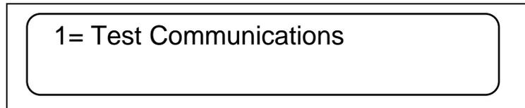
While in the second SETUP screen, pressing 1 will test the communications with another controller if they are interfaced together. If there is no communications, the messages "No Data Received" and "No Data Sent" will be seen.
