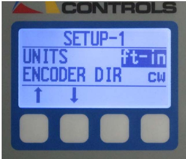
4. With the UNITS field highlighted, press any number Key to scroll between mm, in and ft-in.
