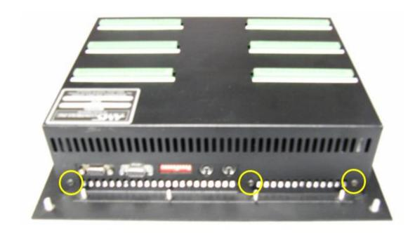
3. Remove the 3 screws on the top of the controller circled in yellow in Figure 4.
