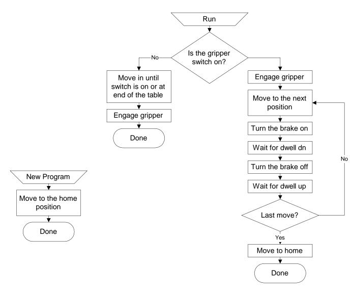
When part information is programmed, and the RUN button is pressed the gripper will try to find the part in the forward direction. As long as the programmed part is shorter than the clearance position, the part will be processed. If the part is physically longer than the clearance position, the gripper must be jogged back to allow the part to be accepted. This must be done on the first part of that length, and the machine will readjust itself for the remaining parts.
