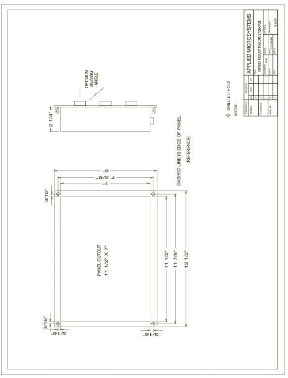
Figure B-1. Panel Mount Mounting Dimensions
