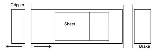
When part information is programmed, and the RUN button is pressed the gripper will try to find the part in the forward direction. As long as the programmed part is shorter than the clearance position, the part will be processed. If the part is physically longer than the clearance position, the gripper must be jogged back to allow the part to be accepted. This must be done on the first part of that length, and the machine will readjust itself for the remaining parts.
