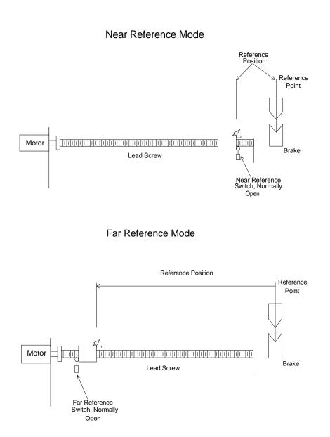
The switch for a NEAR REFERENCE MODE must be normally open and remain closed as long as the Gripper is on the switch or closer to the reference point than the switch. The switch for a FAR REFERENCE MODE must be normally open and remain closed as long as the Gripper is on the switch or farther away from the reference point than the switch.
