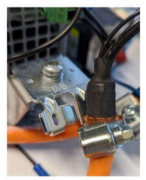
Looking at the motor side of the cable, there is a shield wire terminated with a ring connector. This connector must be connected to the case of the motor via the terminals inside the head of the connector plug. There are two terminals in the head, one for the motor cable, and one for the resolver feedback cable. Some motor/cable combinations have screw on connections at the motor. No additional shield terminations need to be made in these cases.
